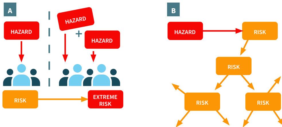
Figure 1: Simplified conceptual diagram explaining (a) compound risks – where more than one event can occur to increase overall risk and (b) cascading risks – where one risk can influence or lead to another risk or series of risks indirectly. Worked examples can be found in the full report.
